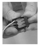
3. Carefully remove the grommet from the water bath cover.
